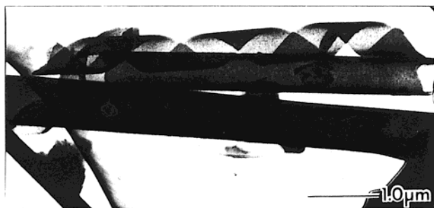
Figure 2. TEM picture of the xerogel 1 prepared from acetic acid (negatively stained with \text{UO}_2^{2+} ).
