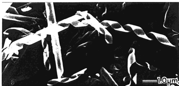
Figure 4. SEM picture of the silica obtained from the 1 + acetic acid gel after calcination.
